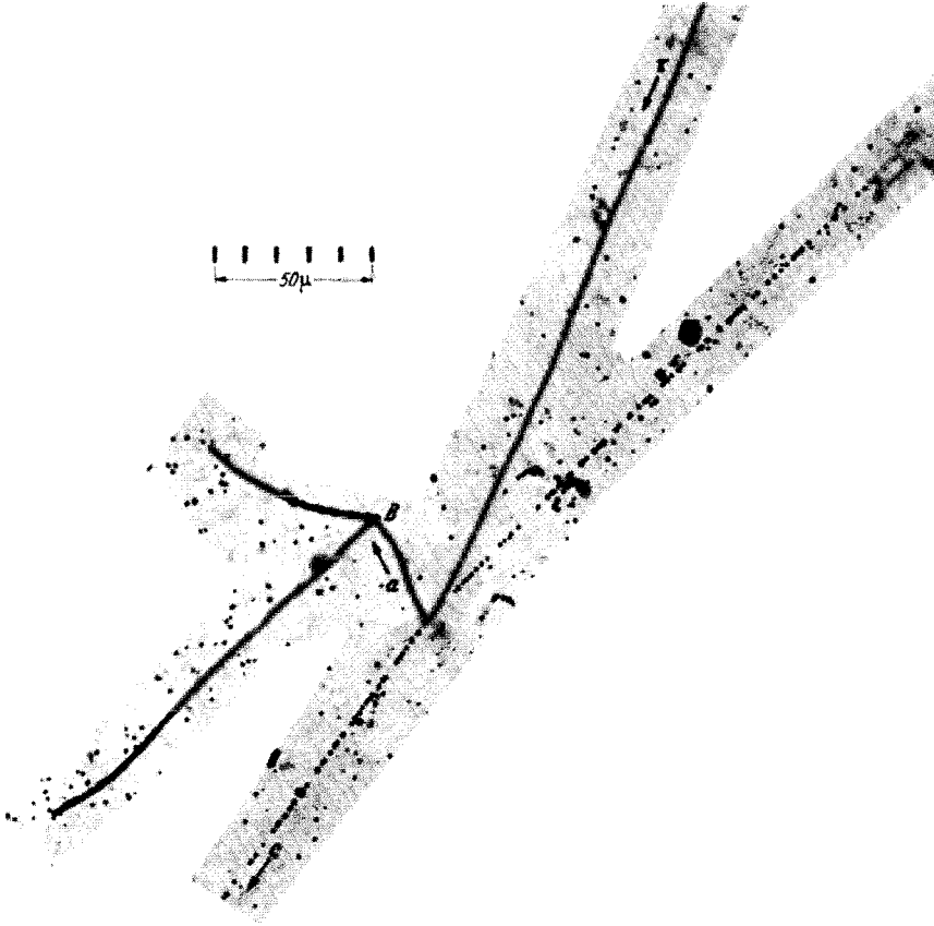
Figure 1.9 K^+ , entering from above, decays at A: K^+ \rightarrow \pi^+ + \pi^+ + \pi^- . (The \pi^- subsequently causes a nuclear disintegration at B). [Reprinted by permission from C. F. Powell, P. H. Fowler, and D. H. Perkins, The Study of Elementary Particles by the Photographic Method (New York: Pergamon, 1959). First published in Rep. Prog. Phys. 13 , 384 (1950).]
